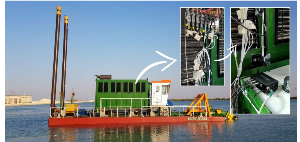
Installation of mDAQ in Dredger
