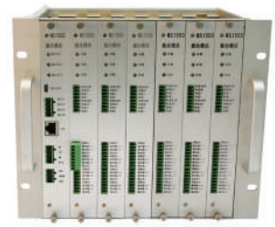
Wired Vibration Monitoring System
