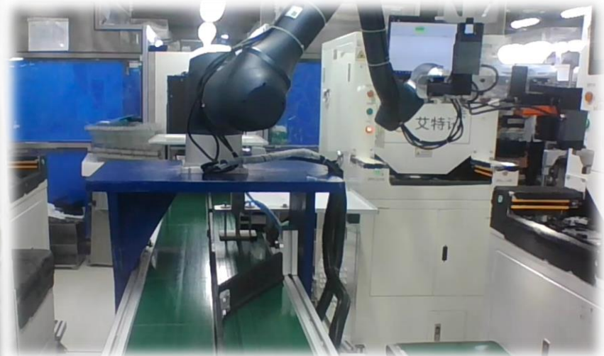
Mobile Phone Testing using Vision - Foxconn
