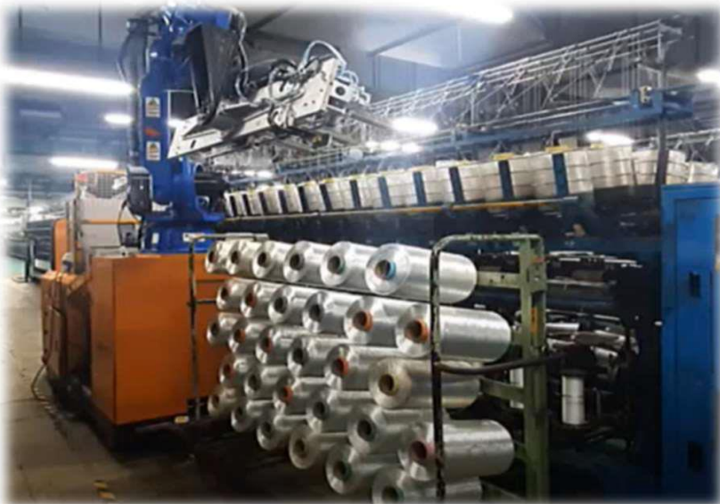
Vision based Bobbin Pick and Place - SRF
